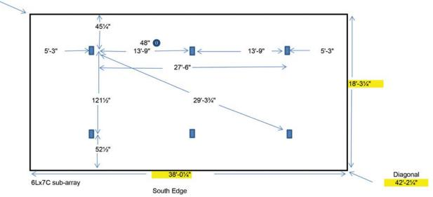
For this 6Lx7C example (6 panels high in landscape by 7 panel columns wide), the 18'-3¼" is the **north-south distance** of the array projected onto the ground. The **east-west dimension** of the array is 38'-0¼".
